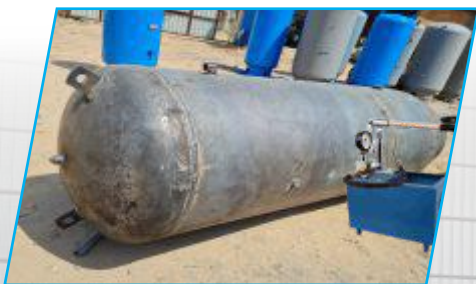
Hydro Testing upto 70 Kg/cm 2 Pressure
