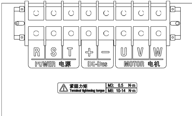
e) Schematic Diagram of Terminals (380V, 45kW-110kW)
